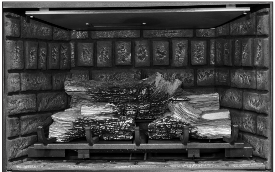
Figure 47: Place both the left and right mid logs in the middle of the air deflector. Make sure the bottom holes align with the pins in the air deflector.
