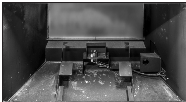
Figure 45: The rear liner can now be removed. Use a vacuum to clean up the bare firebox if needed.
