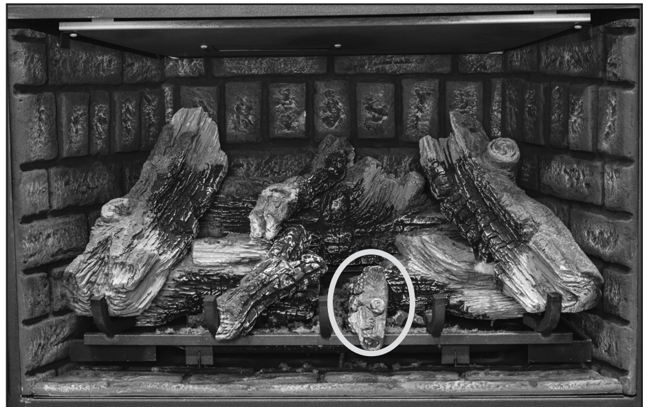
Figure 53: Place the center front chunk log on the log grate, close to the center, with the front edge resting on the right mid log.
