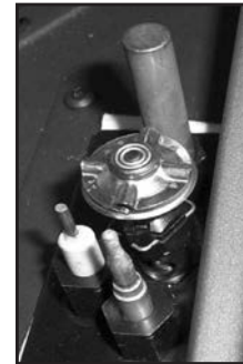
Figure 10: Proper Pilot Position
