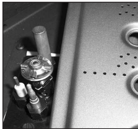
Figure 15: Ignitor assembly beside the burner.
